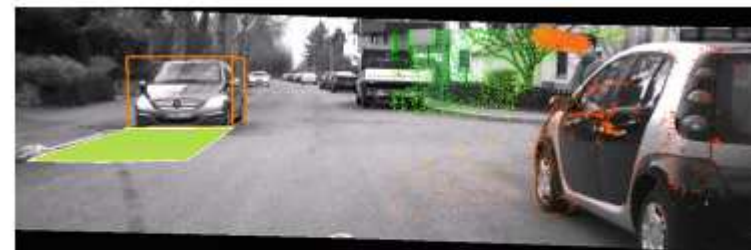
Fig. 29.4 One second before the collision. The camera system has estimated the motion state of the oncoming car, and, at the same time, has detected the crossing pedestrian
